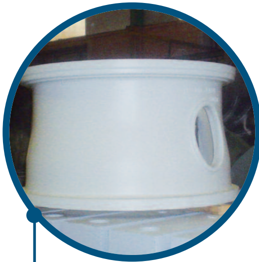
Blade Adaptor Power 2MW 2 tons EN GJS 400-18U LT
